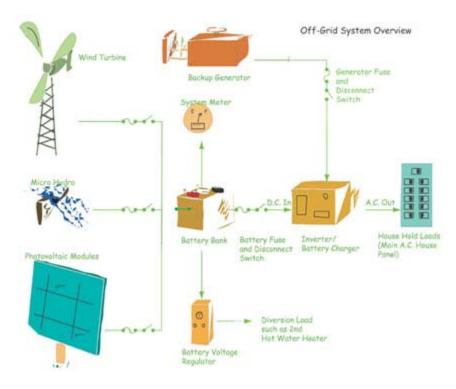
All off-grid systems work much in the same fashion. Collect energy from a renewable source (wind, sun, and/or stream), convert it to electricity and store the energy, usually in a battery bank. When we
